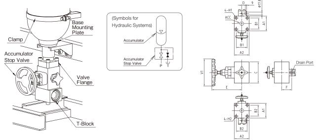
The above accumulator stop valve shows the shape of 6080HFACC3210NS.
