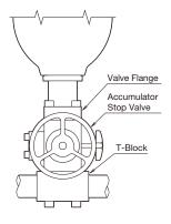
Connection using Acc. Stop Valve and T-Block
