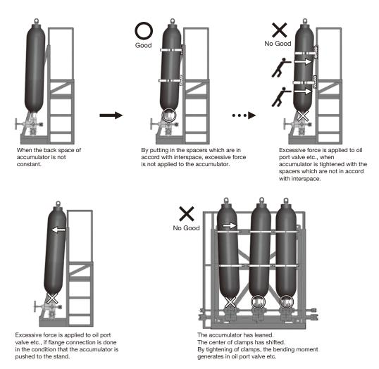
If there is no appropriate interspace between the accumulator and the stand, do not push the accumulator to the stand by force, but redo construction. If it is fixed by force, load may be applied to the piping part or the oil port valve, and it may become the cause of failure or leakage.
