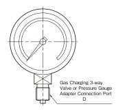
※ Pressure Gauge Adapter 40 MPa and 60 MPa pressure gauges come with a pressure gauge adapter.
