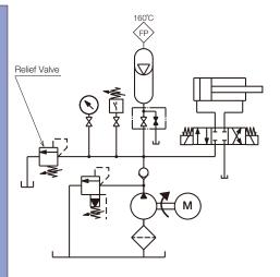
1) Find the required oil volume to be discharged from accumulator Vw (required cylinder oil amount).
