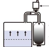
Gas Relief And Charge Valve With Sensor
