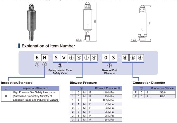
\* Predetermined pressure should be 1.1 times or more of the circuit pressure and less than maximum allowable working pressure of accumulator or other devices.
