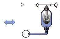
When working fluid from the pump is taken in the oil port side of the accumulator, it pushes the special fluid in the bladder to the next place.
