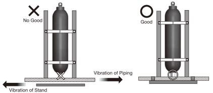
Vibrations of Accumulator and Piping are different
