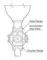
Connection using Acc. Stop Valve and Counter Flange
