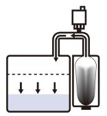
As the fluid level in the tank drops, Dynaclean supplies air to the tank. The Dynaclean bladder contracts.
