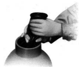
Bladder Replacement Job
