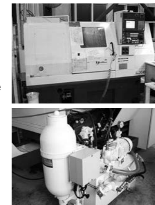
NC Lathe with oil hydraulic unit assembling accumulator for suppressing hydraulic pump electricity consumption.
