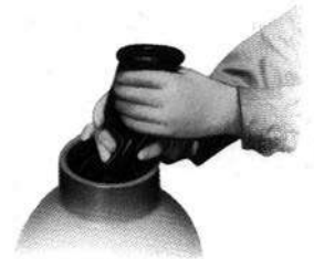
Bladder Replacement Job
