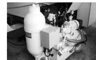
NC Lathe with oil hydraulic unit assembling accumulator for suppressing hydraulic pump electricity consumption.
