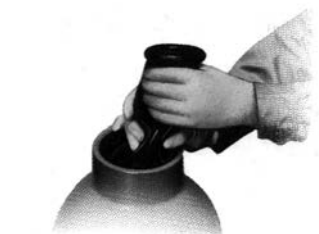
Bladder Replacement Job
